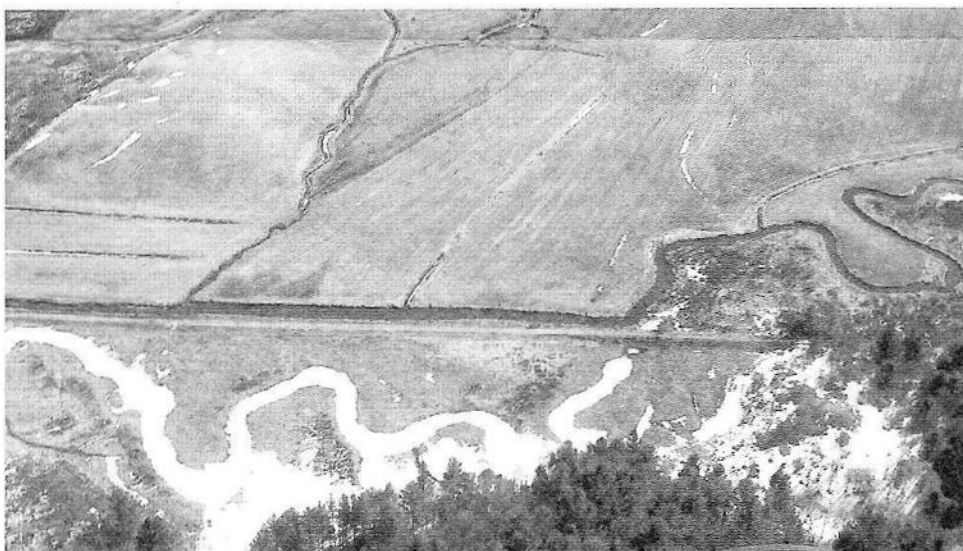
Aerial photo of a floodplain restoration site along Black Creek in Bakersfield. The photo shows a channel that was straightened in the past, and the historic meandering channel, which is covered in snow.
